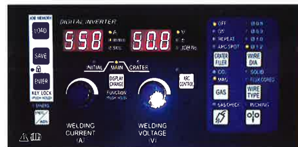
Figure 2 : one knob switch to wire speed display
